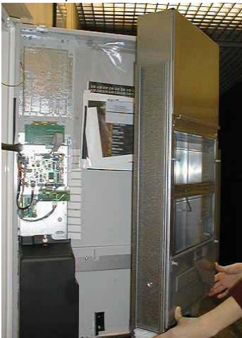
Slide the stirrers still hold together with the packing band along the guide track and, once they have reached the end of the guide, rip the band off.
